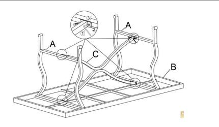
Attach Connector(C) between Legs(A) using Bolts( $\Im$ ) and Washers( $\Im$ ) with Allen Key( $\Im$ ) as pictured above.
