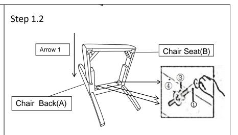
Put the Chair Back(A) onto a flat table or panel. Align the positioning dowels on the Chair Seat(B) with the mounting position located on the Chair Backpanel and Chair-Seat panel.
