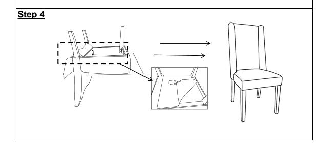
Place the Seat Base Cover(D) back as shown in picture.
