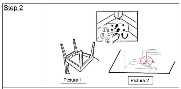
Next, place the chair onto the side of a table as seen in Picture 1. You will now have the chair bottom and all 4-legs facing skywards. Insert each front leg completely vertically into each seat frame corner. PRESS FIRMLY DOWN with your hand until there is no gap.
