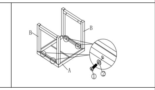
Open the carton and place all the parts onto a clean, non-marring surface. Attach the Table Legsl(B) to Table Top(A)using Hardware((1,2)) with Allen Key((3)) as shown in Picture .
