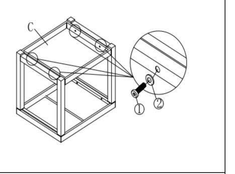
Attach the Table Shelf(C)between the two Table Legs(B) using Hardware((1,2)) with Allen Key((3)) as shown in Picture.
