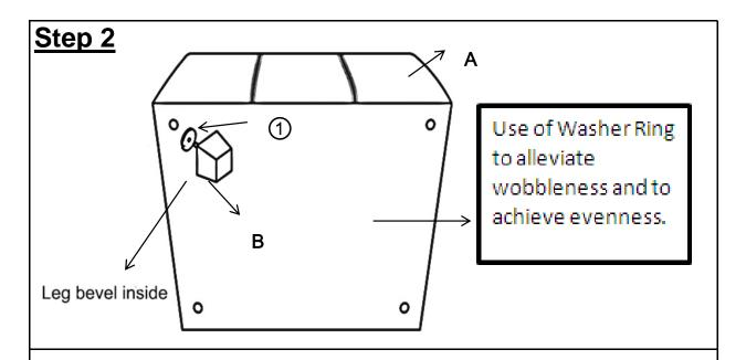
Install the first leg(B) into the bottom of the Storage Ottoman(A) by placing 1 (ONE) piece of Washer Ring on the threaded stem. The use of Washer Rings improves tightness and security of leg after assembly.
