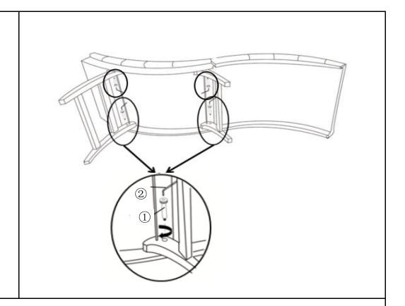
Fixed the leg with Bolts(1), with Allen Wrench(2), as shown, in order to ensure the product stability.
