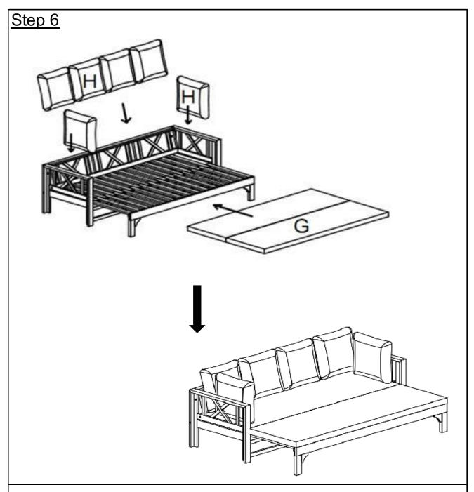
Place Extendable Seat Cushion(G) and Back Pillows(H) onto the Daybed as shown in above picture.
