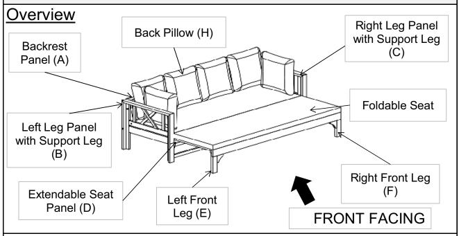
This Daybed has multiple parts and may require up to 30 minutes to assemble. To give you an overview of the Daybed, the above picture is to help you put the various parts into perspective. Please read through the instructions below to familiarise yourself with the parts and steps before assembly.
