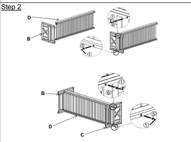
With assistance from your adult partners, attach Left Leg Panel with Support Leg(B) to Extendable Seat Panel(D) using Screw(5) and Screw(6) with Allen Wrench(1) as shown in above picture.
