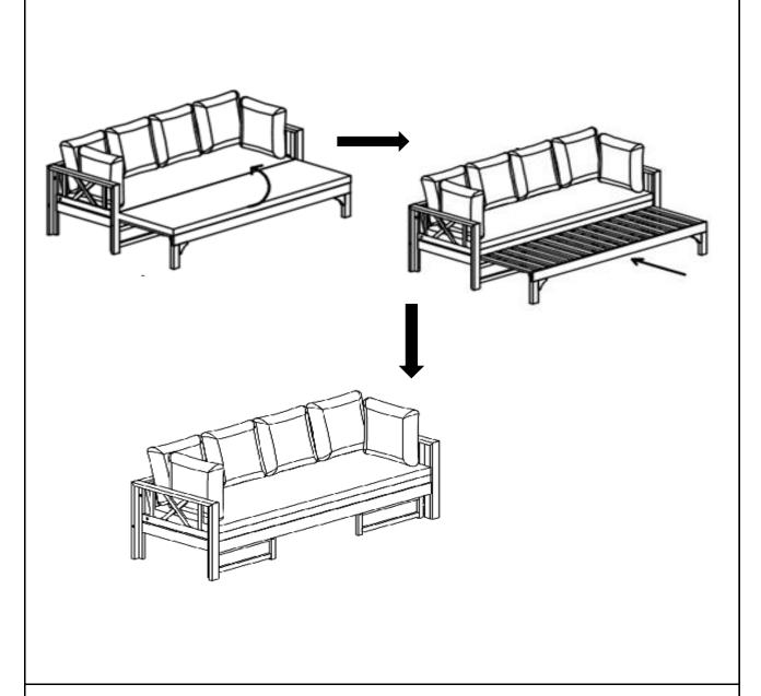
Fold Foldable Seat Cushion(G) in the direction of the arrow and then, push the Extendable Seat Panel(D) to shorten the Daybed as shown in above picture.
