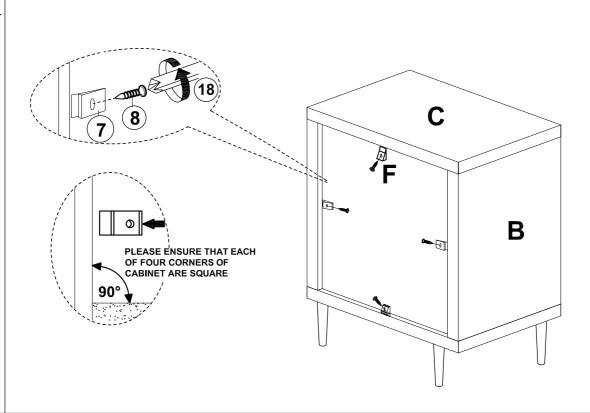
Use Screw Driver (18) to affix Backply Stoppers (7) and Flat Head Screws (8) in the location on Back Panel (F) as shown.
