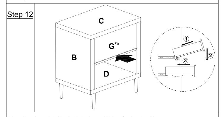
Place the Drawer into the Nightstand assembly by aligning the rails.
