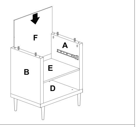
Slide the Back Panel (F) to Right Side Panel (A) and Left Side Panel (B) by inserting it into the grooves as shown.
