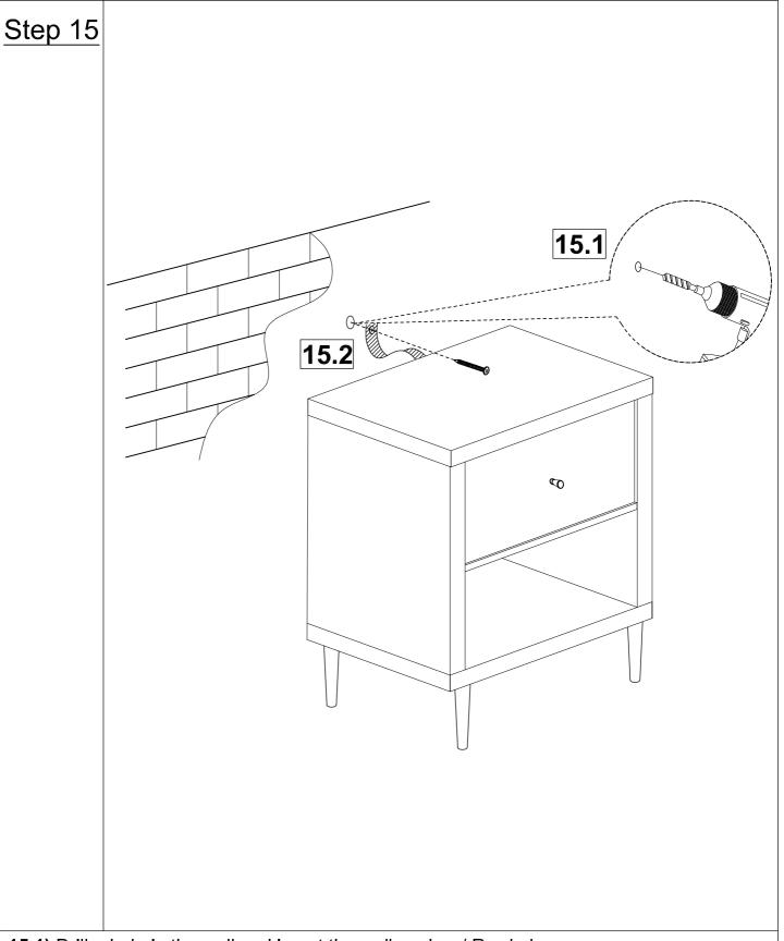
15.1) Drill a hole in the wall and insert the wall anchor / Rawl plug.
