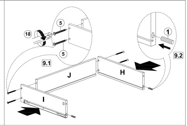
**9.1)** Attach Drawer Right Panel (H) & Drawer Left Panel (I) to Drawer Back Panel (J) as shown-notice the grooves on each panel is at the bottom. Use Flat Head Screws ) to fasten side panels to back panel.
