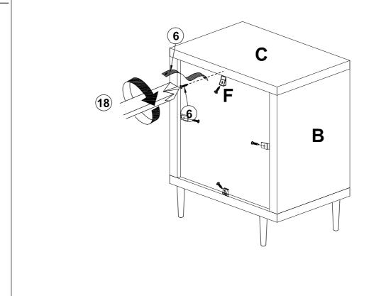
Insert a screw through the Strap (6) at the marked sticker area on back side edge of Top Panel (C) and drive in the screw using a Screw Driver (18).
