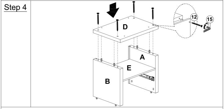
Attach Bottom Panel (D) to Right Side Panel (A) & Left Side Panel (B) via the wood dowels respectively. Use Allen Head (12) to fasten side panels to bottom panel using Allen Wrench (15).
