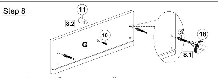
**8.1)** Use a screw driver (18) to screw Cam Bolts (3) into the mounting positions on the inside face of Drawer Front (G) as shown.
