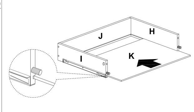
Slide the Drawer Base (K) into the grooves on Drawer Right Panel (H), Drawer Back Panel (J) and Drawer Left Panel (I).
