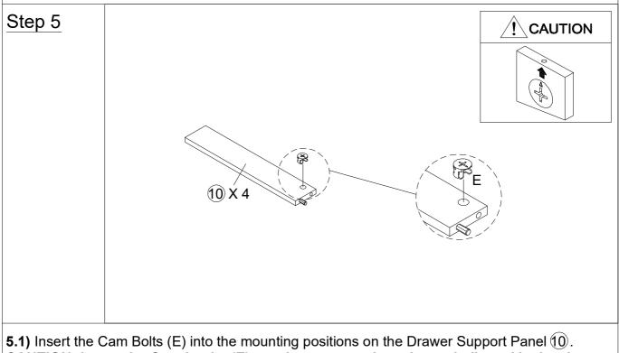
CAUTION: Insert the Cam Locks (E) per the correct orientation as indicated in the above picture.
