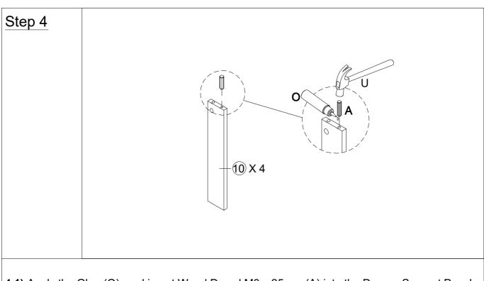
**4.1)** Apply the Glue (O), and insert Wood Dowel M6 x 25mm (A) into the Drawer Support Panel (10) using the Hammer (U).
