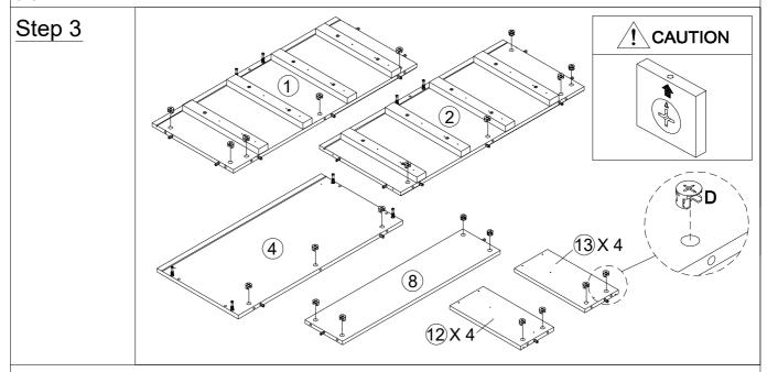
**3.1)** Insert the Cam Locks (D) into the mounting positions on the Left Side Panel (1), Right Side Panel (2), Top Panel (4), Support Panel (8), Left Drawer Side Panel (12) and Right Drawer Side Panel (13).
