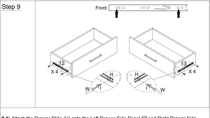
**9.1)** Attach the Drawer Slide (H) onto the Left Drawer Side Panel (2) and Right Drawer Side Panel (3) using the Screw M4 x 14mm (I) with the Screwdriver (W). Note: There are pre-existing mounting positions on the panels to attach the Drawer Slide (H).
