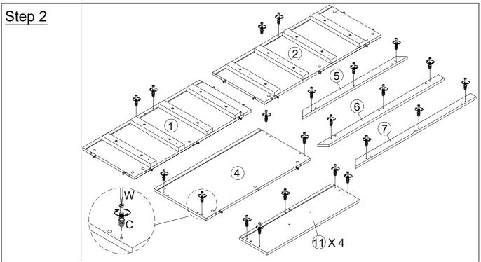
**2.1)** Insert the Cam Bolts (C) into the mounting positions on the Left Side Panel (1), Right Side Panel (2), Top Panel (4), Top Frame (5), Left Side Frame (6), Right Side Frame (7) and Drawer Front (1) using the Screwdriver (W).
