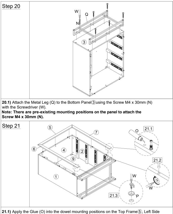
**21.1)** Apply the Glue (O) into the dowel mounting positions on the Top Frame(5), Left Side Frame(6) and Right Side Frame(7).
