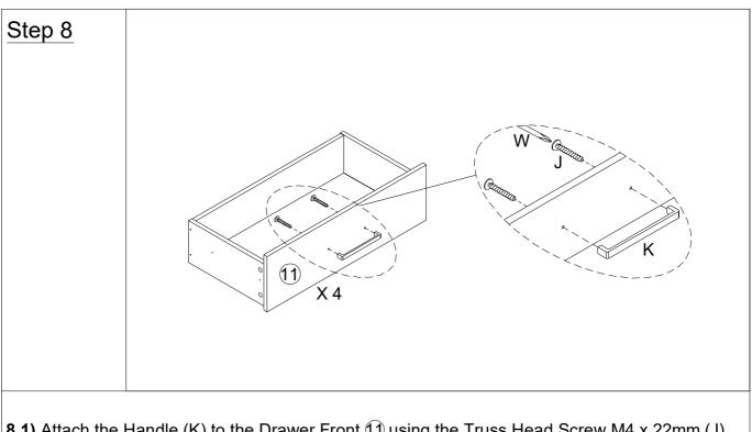
**8.1)** Attach the Handle (K) to the Drawer Front (1) using the Truss Head Screw M4 x 22mm (J) with the Screwdriver (W).
