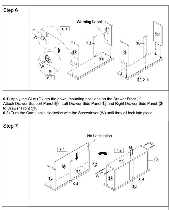
**7.1)** Insert the Drawer Panel 15 along the grooves on Drawer Front 1, Left Drawer Side Panel 2 and Right Drawer Side Panel 3.
