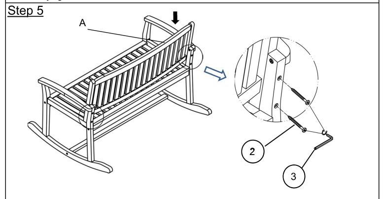
With the help from your partner, turn the finished part in step 5 right side up. Attach Backrest Panel (A) to Right Leg Panel (D) and Left Leg Panel (C), secure by using Screw ((2)) and Allen Wrench ((3)).
