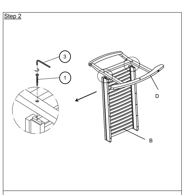
With the help from your assistance, place the Seat Panel (B) with its one side face skywards onto a clean, soft surface to avoid any scratches or damages to the product. Align the tenon of Seat Panel (B) into the Mortise of Right Leg Panel (D) as shown above. Then, affix the Seat Panel (B) with Right Leg Panel (D) by using Screws (1) and Allen Wrench
