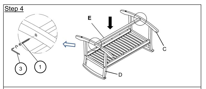
Attach the Leg Support Bar (E) to the Right Leg Panel (D) and Left Leg Panel (C) by using Screws(1) with Allen Wrench(3).
