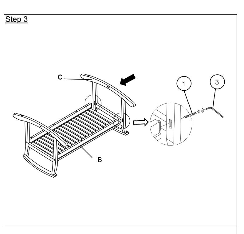
With the help from your partner, place the assembled part on step 2 to the Left Leg Panel (C) as shown in picture above.
