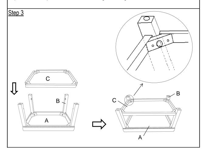
With assistance from your adult partner, Carefully place the Shelf(C) into the grooves on the Legs(B). Make sure the Shelf(C) four corners get stuck into the grooves on the Legs as above shown.
