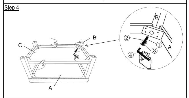
Two adults are recommended for this step. Each one to hold the Shelf(C) on a side with a hand, and at the same time, assembly with other hand.
