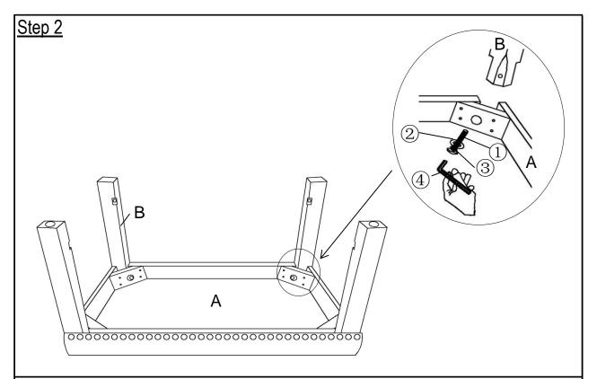
Insert Leg(B) into the groove of underside of Bench Seat(A).
