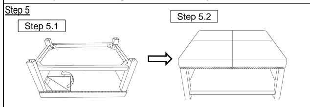
**5.1)** Seal the non-woven bottom cover back on the underside of the Bench.
