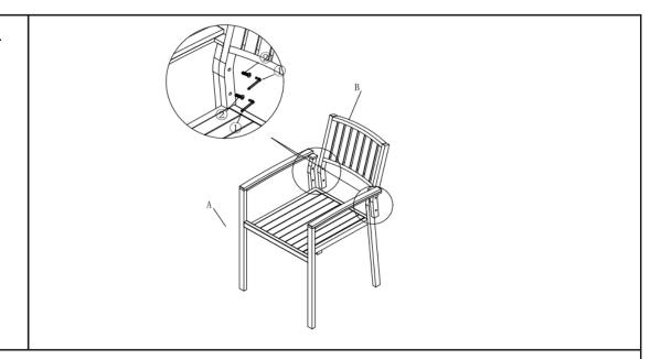
Attach Backrest(B) to Seat(A) using Bolts(1) with the Allen Wrench(2) as shown above. Do not fully tighten the Bolts.
