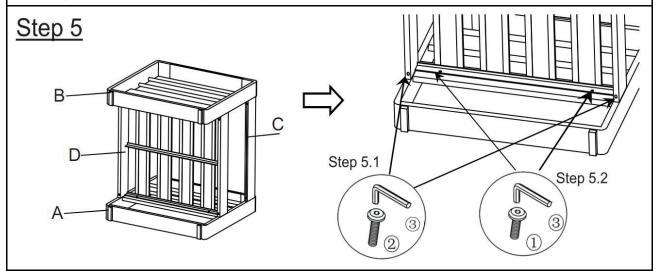
5.1)Attach the Right Side Panel(B) to the Seat(D) using Bolts(2) and the Allen wrench (3) as shown in the picture. 5.2)Attach the Right Side Panel(B) to the Seat(D) using Bolt(1) with Allen wrench (3) as shown in the picture. Place the chair upright and test for stability.
