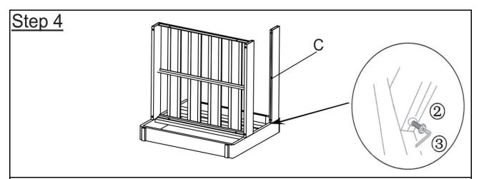
Connect the Back Support Bar (C) to the Left Side Panel (A) using an inner hexagon Allen wrench(③) and bolt (②) as shown.
