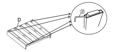
As shown above, use an inner hexagon Allen wrench (③)to remove the plastic plug (inserted to prevent aluminum deformation) from the four ends of the seat (D). If necessary, please keep the plastic plug for repacking.
