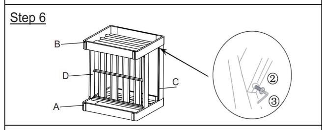
As shown, bolt(2) and connect the Back Support Bar (C) to the right panel(B)with an inner hexagon Allen wrench (3).
