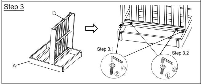
3.1)Attach Seat(D) to the Left Side Panel(A) using Bolts(2) and the Allen wrench (3) as shown in the picture. 3.2)Attach Seat(D) to the Left Side Panel(A) using Bolt(1) with Allen wrench (3) as shown in the picture. Do not fully tighten the Bolts at this time.
