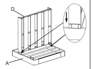
Open the carton and place all parts on a clean, non-marring surface. Insert seat (D) into the Left Side Panel (A) as shown.
