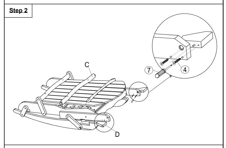
Insert Wooden Dowel on Support Corners (D) into hole on the leg of Foldable Seat and Backrest (C) then secure using Screws (4) and Screwdriver (7) as above picture.
