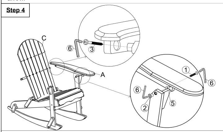
Put tenon of Backrest Support of Foldable Seat and Backrest (C) into the hole of Right Armrest (A) using Screw (③), Allen Wrench (⑥). Attach Right Armrest (A) to Foldable Seat and Backrest (C) using Bolt (①), Sleeve Nut (②), Plastic Washer (⑤) and 2 Allen Wrench (⑥). Repeat the same process with the Left Armrest (B).
