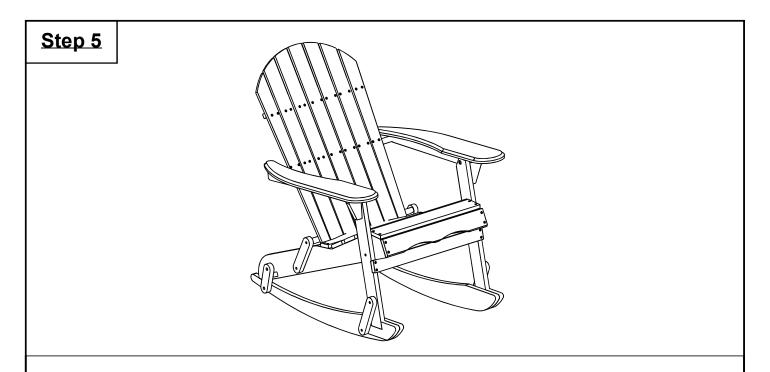
In a sequential manner, tighten all Bolts and Screws at all joints until fully locked into position.
