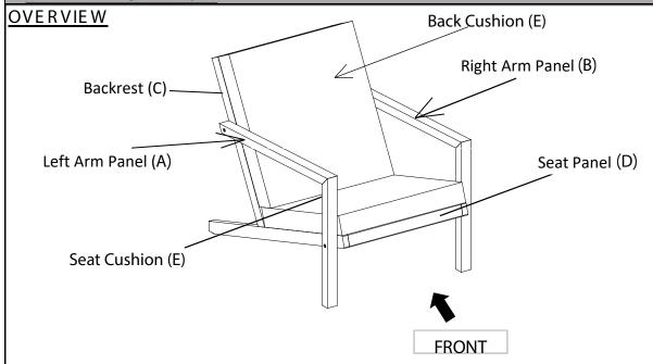
This Counter Chair has multiple parts and may require up to 30 minutes to assemble. To give you an overview of the Counter Chair parts, the above picture is to help you put the various parts into perspective. Please read through the instructions herebelow to familiarise the parts and steps before assembly.
