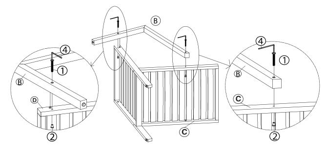
Attach Right Armrest (B) with the assembled frame in step 2 as shown in picture.
