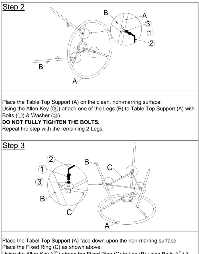
Using the Allen Key (2) attach the Fixed Ring (C) to Leg (B) using Bolts (1) & Washer (3).
