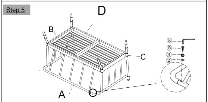
Attach Right Arm Panel(C) to Backrest Panel(A)using Washers(2), Spring Washers(3) and Bolts(5) with Allen Key(8) as shown.
