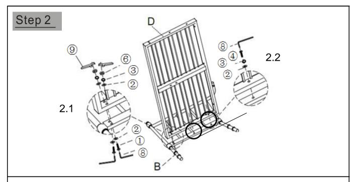
Place Left Arm Panel(B) with its one side face skywards onto a clean, soft surface to avoid any scratches or damages to the product.
