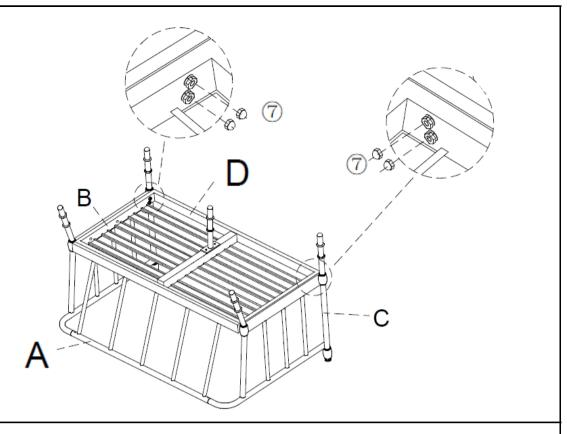
Now, fully and securely, tighten all nuts, at all joints. Put the Nut caps( $\Im$ ) on the Nut as show in above pictures.
