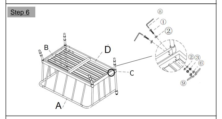
Attach Seat Panel(D) to Right Arm Panel(C) using Bolts(1), Washers(2), Spring Washers(3) and Nut(6) with Allen Key(8) and Wrench(9).
