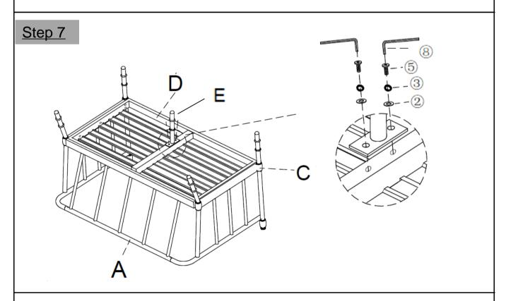
Attach Middle Leg(E) to Seat Panel(D) using Washers(2), Spring Washers(3) and Bolts(5) with Allen Key(8).
