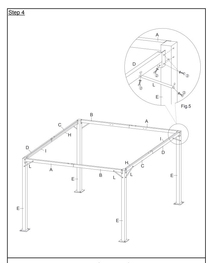
Attach Crossbars(C) to Main Pillars(E) using Bolts(②) with Wrench(③).
