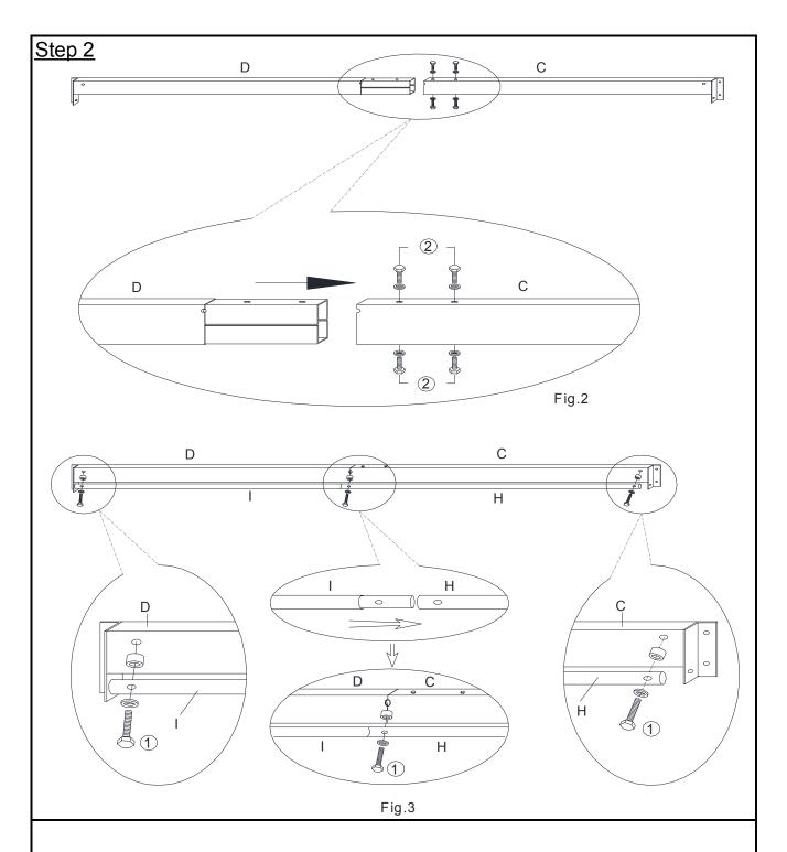
Attach Crossbars(C) to Crossbars(D) using Bolts(2) with Wrench(3). (See Fig. 2)
