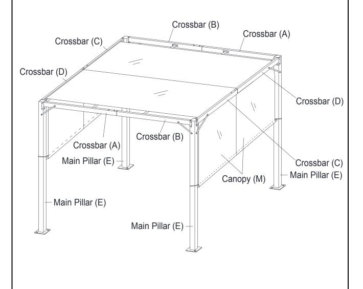
This Gazebo has multiple parts and may require up to 3-4 hours to assemble. To give you an overview of the Gazebo parts, the above picture is to help you put the various parts into perspective. Please read through the instructions below to familiarise yourself with the parts and steps before assembly.
