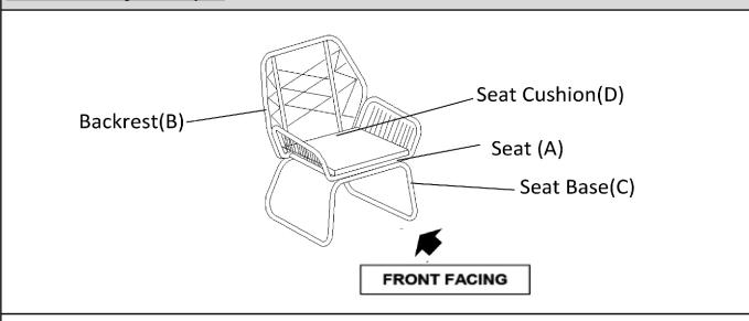
This Chair has multiple parts and may require up to 30 minutes to assemble. To give you an overview of the Swivel Chair parts, the above picture is to help you put the various parts into perspective. Please read through the instructions below to familiarise yourself with the parts and steps before assembly.
