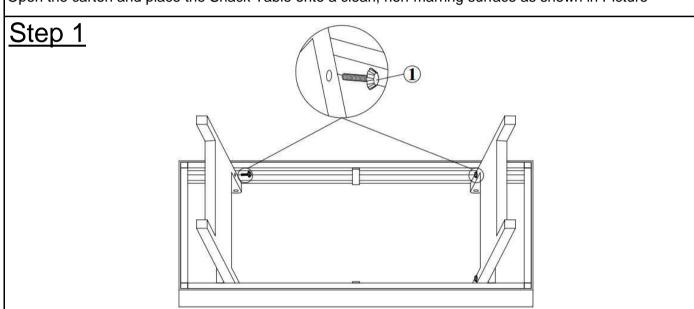
Attach the Table Leg onto the surport bar on the table top using Bolt (1) as above picture show. Fully tighten the Bolts.
