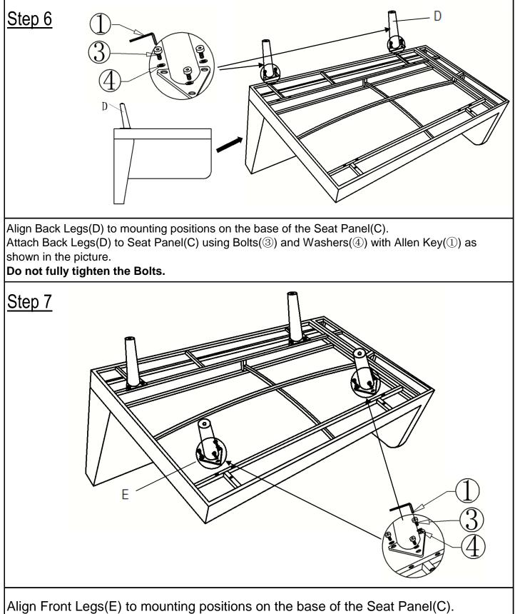
Attach Front Legs(E) to Mounting positions on the base of the Seat Panel(C). Attach Front Legs(E) to Seat Panel(C) using Bolts( $\Im$ ) and Washers( $\Phi$ ) with Allen Key( $\square$ ) as shown in the picture.
