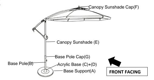
This Canopy Sunshade has multiple parts and may require up to some 30 minutes to assemble. To give you an overview of the Canopy Sunshade parts, the above picture is to help you put the various parts into perspective. Please read through the instructions below to familiarise yourself with the parts and steps before assembly.
