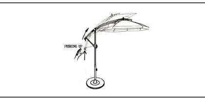
To adjust the Canopy Sunshade angle, push the Curved Support Pole upwardsor downwards until you reach the desired height.
