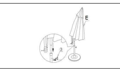
Insert the pole of the Canopy Sunshade(E) into the Base Pole(B) aligning them ounting positions of (E) and (B). Screw-in the Screw With Acrylic Cap(③) by hand into the mounting positions of(E) and (B) to ensure that the pole is tightly secured to the base. Your Canopy Sunshade is fully assembled.
