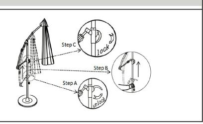
To use the Canopy Sunshade, you need to apply a 3 step process. These are :Step A - First push the lever of the Hand Grip upwards to unlock the CurvedSupport Pole. Step B - Then slide the Hand Grip upwards along the pole about one meterabove the ground. Step C - To lock, pull down the lever of the Hand Grip to lock onto the CurvedSupport Pole into position.
