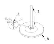
Align the mounting positions of the Base Pole(B) onto Base Support(A) and attach them with Washer(1) and Nut(2) using Wrench(4).
