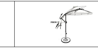
To adjust the Canopy Sunshade angle, push the Curved Support Pole upwardsor downwards until you reach the desired height.
