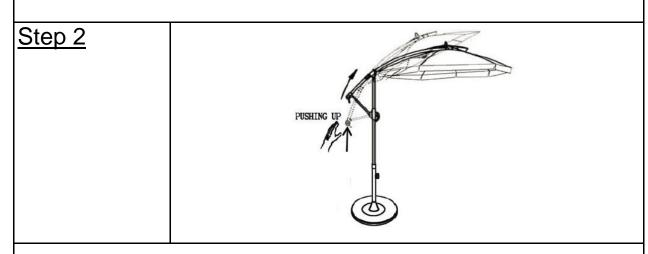
Open the Canopy Sunshade by rotating the Crank clockwise. To close, rotate the Crank counterclockwise.
