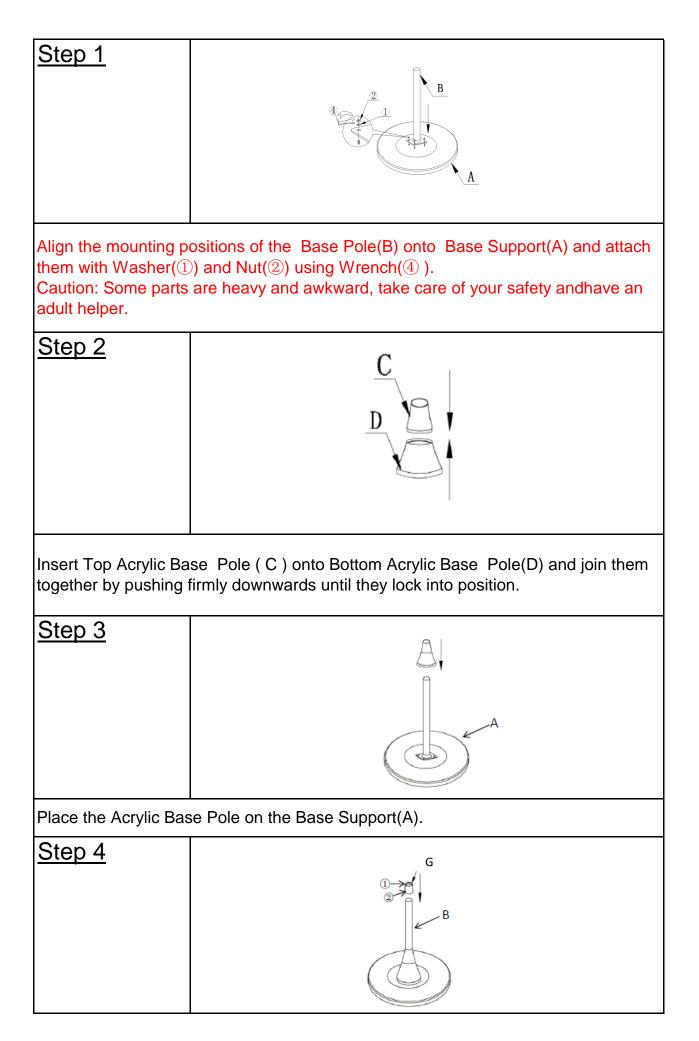
Insert Base Pole Cap(G) onto Base Pole(B).Ensure the label marked "2" is at the bottom.Note: The Base Pole Cap(G) may require additional force to attach completely.If necessary please use a rubber mallet or wooden hammer to gently tap them into place.
