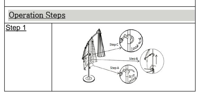
To use the Canopy Sunshade, you need to apply a 3 step process. These are :Step A - First push the lever of the Hand Grip upwards to unlock the CurvedSupport Pole.Step B - Then slide the Hand Grip upwards along the pole about one meterabove the ground. Step C - To lock, pull down the lever of the Hand Grip to lock onto the CurvedSupport Pole into position.
