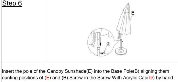
into the mounting positions of(E) and (B) to ensure that the pole is tightly secured to the base. Your Canopy Sunshade is fully assembled.
