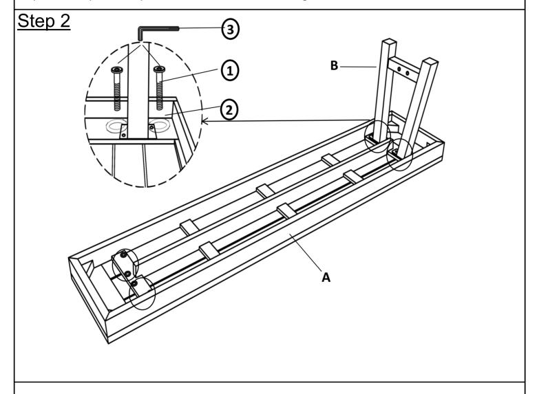
Place the Seat Panel(A) facedown onto a clean, non-marring surface. Attach Iron Legs(B) to Seat Panel(A) using Bolts( $\widehat{1}$ ) and Washers( $\widehat{2}$ ) with Allen Wrench( $\widehat{3}$ ).
