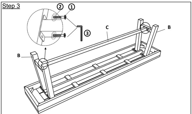
Attach Support Bar(C) to Iron Legs(B) using Bolts(1), and Washers(2) with Allen Wrench(3) as pictured above.
