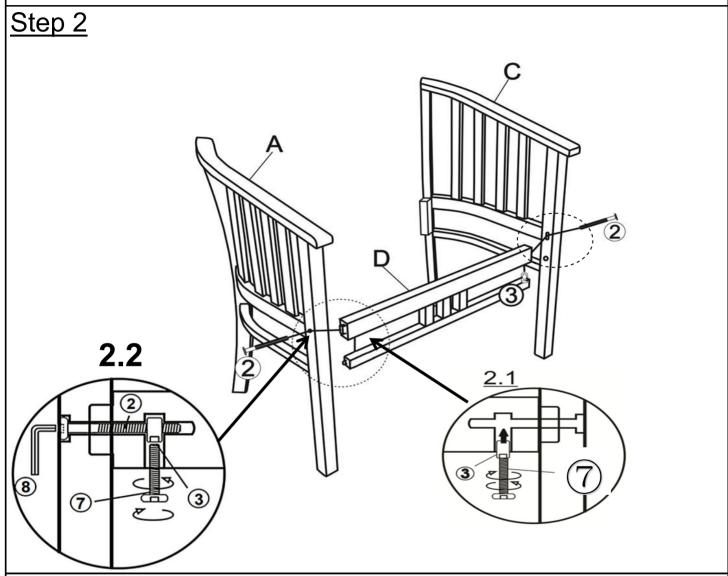
Insert the tenons on Leg Support Bar(D) into the mortises on Left Arm Panel(A).
