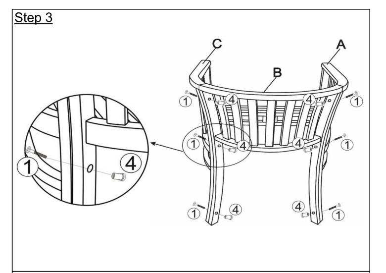
Attach Backrest Panel(B) to Left Arm Panel(A) and Right Arm Panel(C) using Bolts(1) and Sleeve Nuts(4) with Allen Wrenchs(8).
