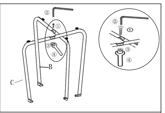
Align the mounting positions of Leg(B) and Leg(C) as shown above, then attach using Bolt(1) and Nut(3) with Allen Key(2) and Spanner(4).
