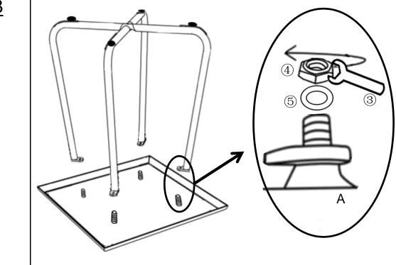
Carefully place the Table Top(A) facedown on a clean, non-marring surface. Align the mounting positions of Legs with Table Top(A).
