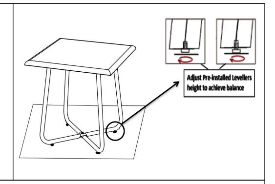
Adjust the Pre-installed Levellers at the base of the Legs until the Chair is level to the ground.
