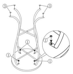
Loosely tighten nuts (①)with the wrench (②), add Pads(③) onto the feet. **Do not fully tighten the Nuts.**
