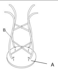
Unfold the Table Leg (B) and align with pre-assembled studs on Table Top(A).
