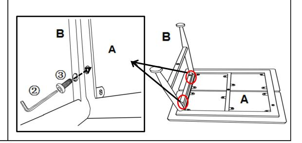
Place the Table Top(A) facedown onto a clean, non-marring surface. Align the mounting positions on the Table Top(A) and the Leg (B). Attach Leg(B) to Table Top(A) using Bolts (③) with Allen Key(②) as shown.
