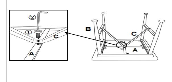
Attach the "V" Shape support(C) into the Table Top(A) using Bolts (1) with Allen Key(2) as shown.
