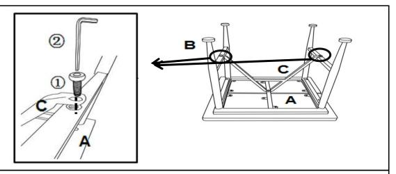
Attach the "V" Shape support(C) into the Legs(B) using Bolts (1) with Allen Key(2) as shown.
