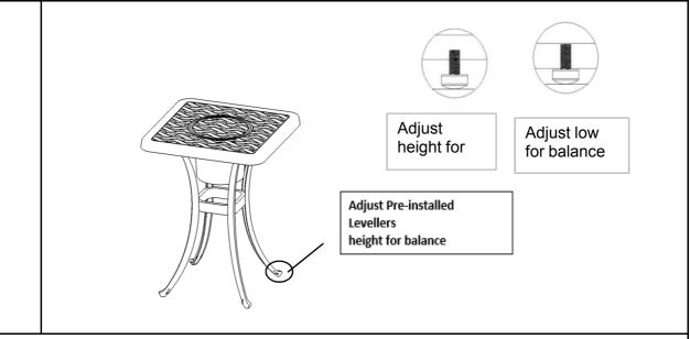
When necessary adjust the Pre-installed Levellers at the end of each Table Leg until the Table is level with the groud.
