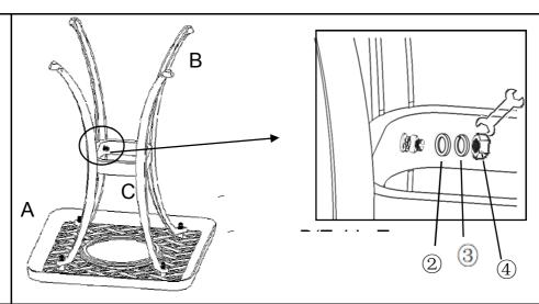
Attach the Central Square Support Ring(C) to Table Leg(B) using Washers(2), Spring Washers(3) and Nuts(4) with the Spanner(7). Repeat the same tightening at all 4 poins of the Legs.
