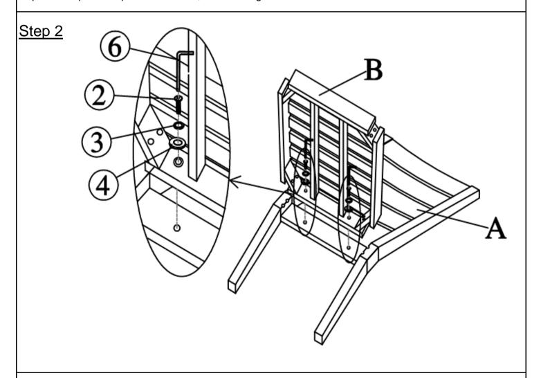
Place the Backrest Panel(A) facedown onto a clean, non-marring surface. Align Seat Panel(B) to Backrest Panel(A) then attach using Bolts(2), Spring Washers(3), and Washers(4) with Allen Wrench(6).
