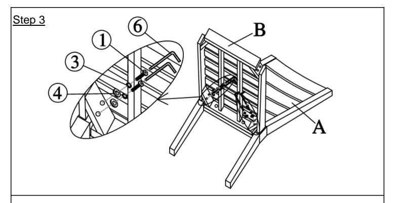
Attach Seat Panel(B) to Backrest Panel(A) using Bolts(1), Spring Washers(3), and Washers(4) with Allen Wrench(6).
