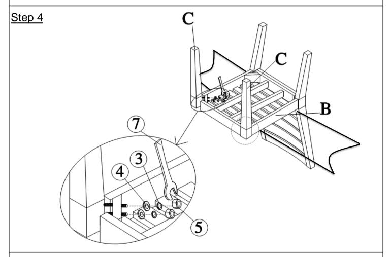
Attach Leg Panel(C) to Seat Panel(B) using Nuts(5), Spring Washers(3), and Washers(4) with Spanner(7).
