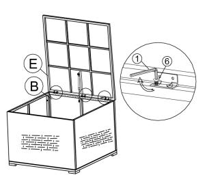
Attach Lid-Top Panel(E) to the Back Panel(B) using Bolt(6) with Allen Key(1) as shown in the picture above.
