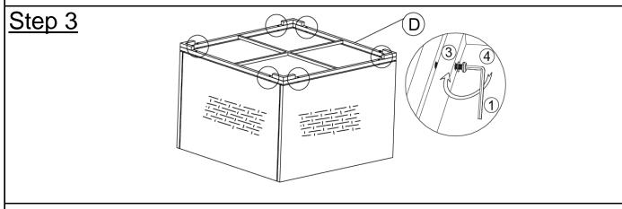
Attach Base Panel(D) to the four Side Panels using Bolts(④) and Washers(③) with Allen Key(①) as shown in the picture above. **Do not fully tighten the Bolts.**
