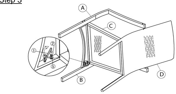
Attach Left Armrest / Leg(B) to Seat(C) using Bolts(2) and Washers(5) with Allen Key(1) as shown in the picture above.
