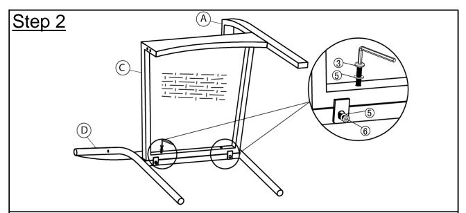
Attach Backrest(D) to Seat(C) using Bolts(3&6) and Washers(5) with Allen Key(1) as pictured above.
