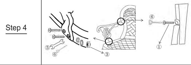
Connect the Right arm(E) and Left arm (F) to Seat Panel (B) using Bolts, Washers, Spring washers and Nuts (6mm)(③).
