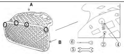
Place the Seat and Backrest panels as shown in above pictorial. Attach the Studs (4)((M8\*40mm) into the contact points on the Chair Back Panel (A) using the Screwdriver (6). Then attach the Seat Panel (B) to the Chair Back Panel (A) using Washers, Spring Washers and Nuts (8mm)(2).
