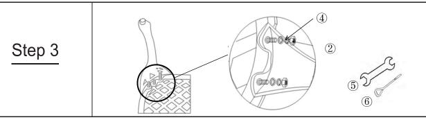
Attach the Studs(4)(M8\*40mm) to the contact points on Chair Seat Panel (B) using the Screwdriver (6).
