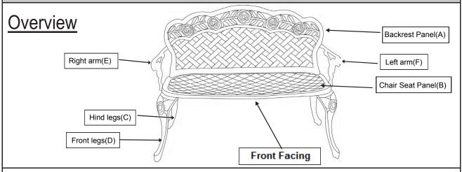
This Chair has multiple parts and may require up to some 30 minutes to assemble. To give you an overview of the 6 parts, the above picture is to help you put the various parts into perspective. Please read through the instructions below to familiarise yourself with the parts and steps before assembly.
