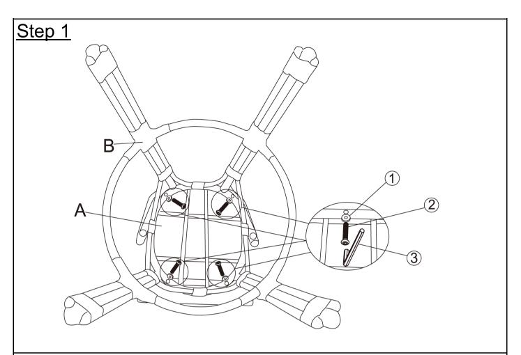
Open the carton and place all the parts onto a clean, non-marring surface. Attach the Leg Base(B) to the Backrest/Seat(A) with Washers(1) and Bolts(2) using the Allen wrench(3) as shown above.
