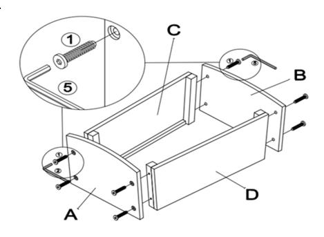
With assistance from your adult partner, attach the Front Panel(A) and the Back Panel(B) to the Left Panel© and the Right Panel(D) using 8 Screws( $\bigcirc$ 1) and the Allen Key( $\bigcirc$ 5) as shown in the above picture.
