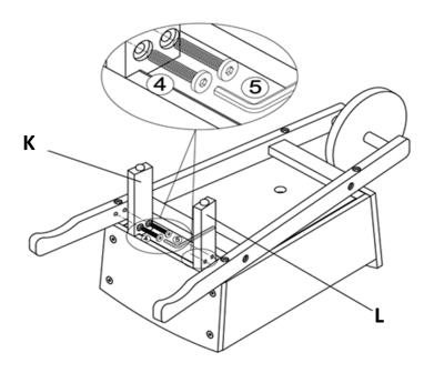
With assistance from your adult partner, place the Left Leg(K) and the Right Leg(L) onto the assembled part in Step 4 as shown in the above picture. Loosely affix by using the Bolts(4) and the Allen Key(5) as shown in the above picture.
