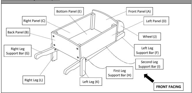
This Planter has multiple parts and may require up to 20 minutes to assemble. To give you an overview of the Planter parts, the above picture is to help you put the various parts into perspective. Please read through the instructions below to familiarise yourself with the parts and steps before assembly.
