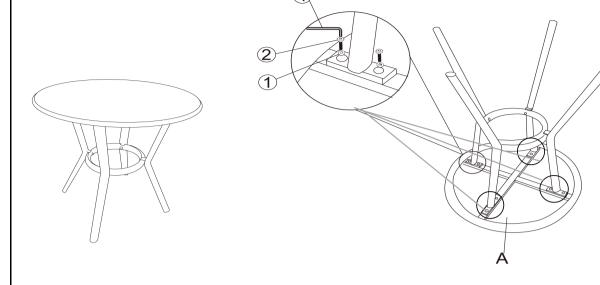
Attach one of the Legs(B) to the Table top (A) with the Bolts(2) and washers (1) using the Allen Key(4) as shown above.
