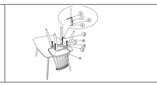
Place the Chair Seat(A) face down as picture on a clean, non-marring table. With assistance from second adult, attach Leg Frame(B) to Chair Seat(A) using Bolts(1), Flat Washers(2) and Spring Washer (4) with Allen Key(3).
