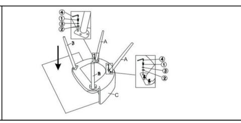
Attach the Back Legs(A) to the Chair Body(C) using the Bolts(1), washers(2) and spring washers(3), with the Allen Wrench(4) as pictured above.
