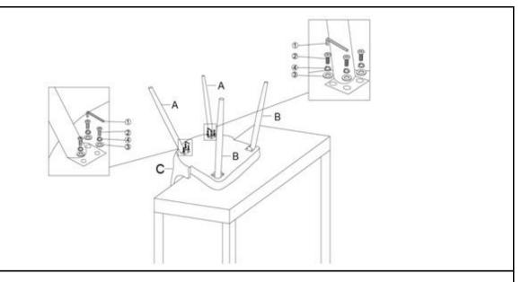
Attach Hind Leg(A) to Chair Seat(C) using Bolts(2), Washers(3), and Spring Washers(4), with Allen Key(1) as pictured above.
