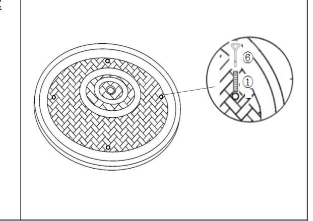
Lay the Table Top(A), facedown, onto a flat, soft, clean surface and lock the mounting positions with bolts(1) by using screwdriver(6). **Need tighten the bolts.**
