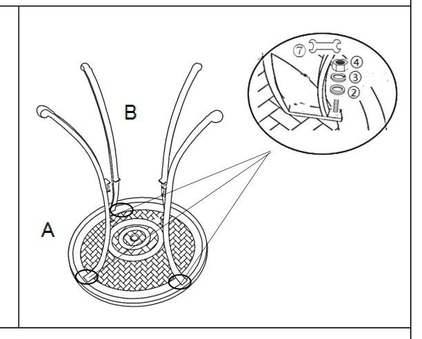
Repeat step 3, attaching the remaining 3 legs to the Table Top(A). At this stage, only loosely tighten the bolts.
