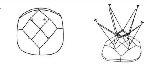
Carefully place the Chair Body (B) upside down on a clean, non-marring table. With assistant from second adult,gently place the Leg Frame(B) onto the Chair Body(A) and align the four mounting positions of both, the Leg Frame(B) onto the Chair Body(A).
