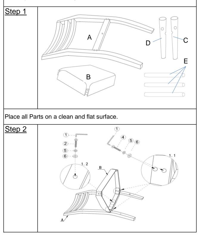
1.1 Install the Seat Cushion (B) using the Allen Wrench (①),Bolts (④), Spring Washers (⑤) and Flat washers (⑥), as pictured above.
