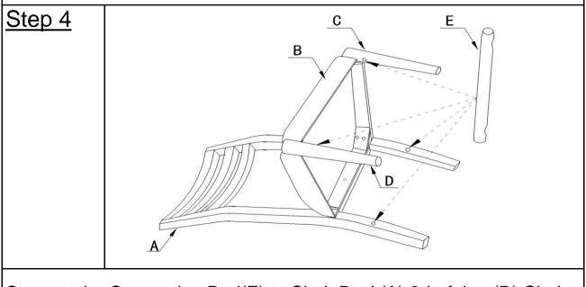
Connect the Connecting Rod(E) to Chair Back(A) & Left Leg(D), Chair Back(A) & Right Leg(C), Right Leg(C) & Left Leg(D) as shown above.
