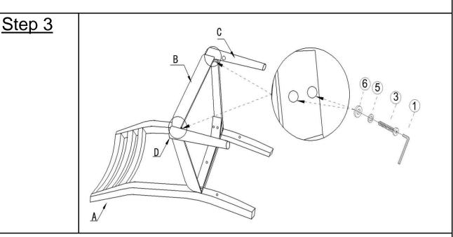
Install the Right Leg (C) and Left Leg(D) using the Allen Wrench (①), Bolts (③), Spring washers (⑤) and Flat washers (⑥), as pictured above.
