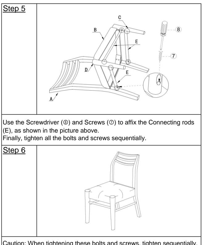
Caution: When tightening these bolts and screws, tighten sequentially. Do not fully tighten one bolt or screw then move to the next one, as this can lead to uneveness.
