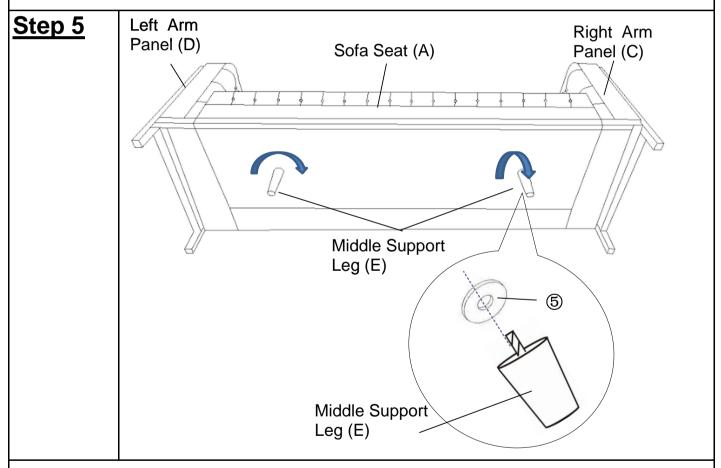
Install the Middle Support Legs(E) with the Washer Ring(5) at the bottom of the sofa on the threaded stem.
