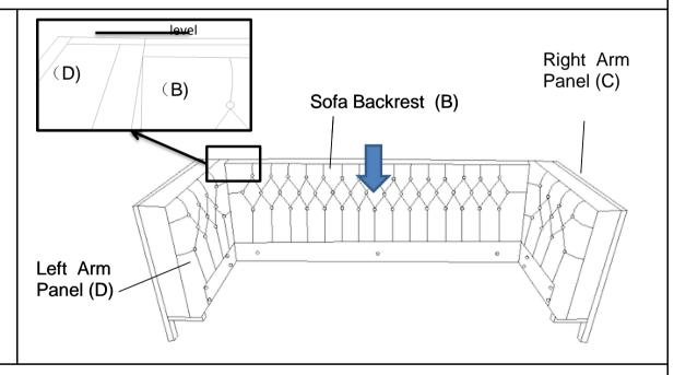
Turn the sofa upright and push the Sofa Backrest (B) downwards until it is fully slotted and locked into position in the Arm Planes.
