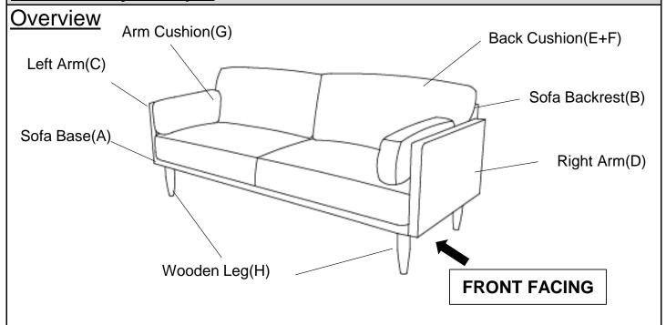
This Sofa has multiple parts and may require about 30 minutes to assemble. To give you an overview of the Sofa parts, the above picture is to help you put the various parts into perspective. Please read through the instructions below to familiarise yourself with the parts and steps before assembly.
