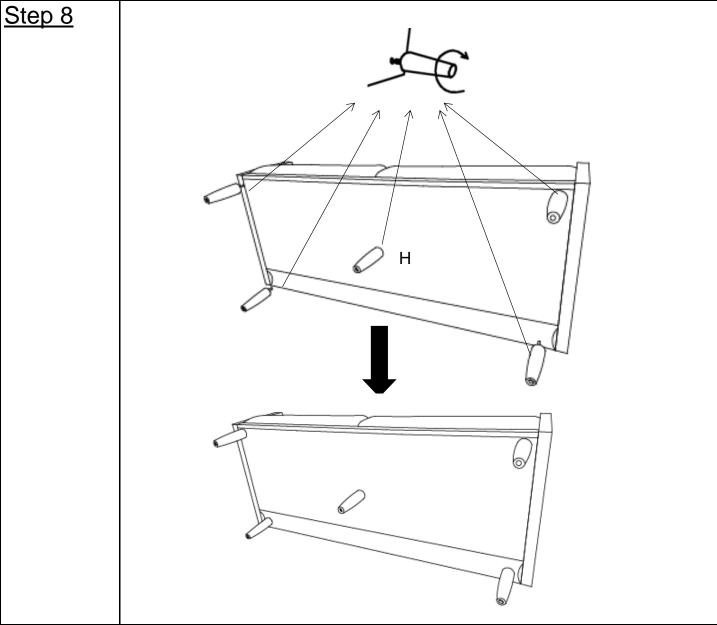
Install the Wooden Legs(H) to the bottom of the Sofa by placing one Gasket(①) on the threaded stem.
