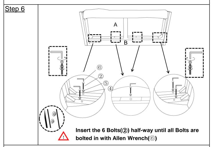
Using the Allen Wrench(⑤) to secure Sofa Base(A) to the front-bottom of Sofa Backrest(B) with the Bolts(②), Spring Ring(⑤)and Washers(④).
