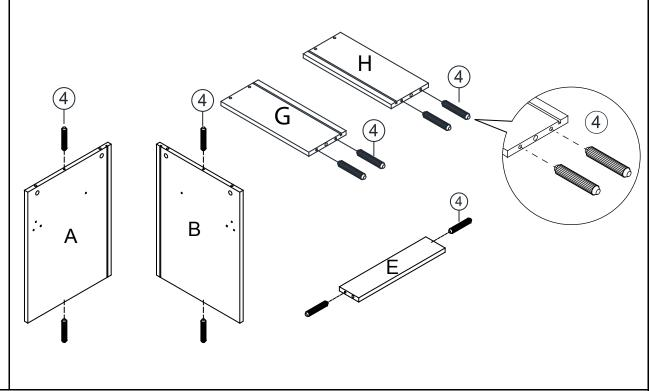
Unpack and place all parts on a clean, non-marring surface. Insert the Positioning Dowels (4)into the mounting positions on the Side Panel Left (A) and Right (B), the Support Panel (E),the Drawer Side Left (G) and Drawer Side Right (H).
