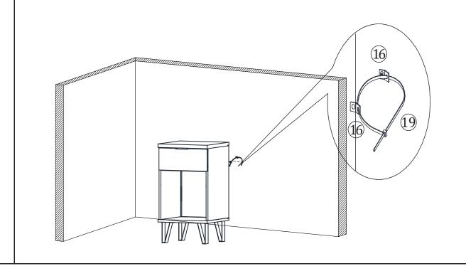
Move the Tall End Table back against wall. Pull the Tipover Restraint Straps(19) through the Metal Brackets(16) on the wall and the Tall End Table one by one, and pull the Tipover Restraint Straps(19) tight.
