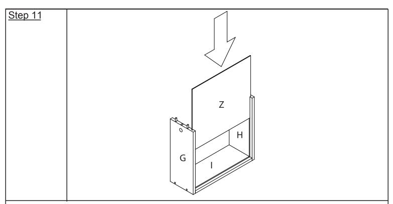
Insert the Drawer Bottom (Z) along the slots on the Drawer Side Right (H) and Drawer Side Left (G).
