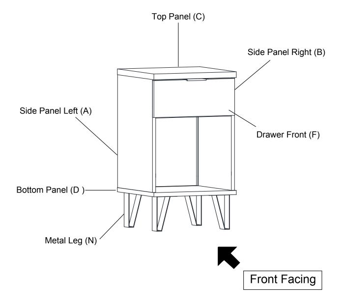
This Tall End Table has multiple parts and may require up to 30 minutes to assemble. To give you an overview of the Tall End Table parts, the above picture is to help you put the various parts into perspective. Please read through the instructions below to familiarise yourself with the parts and steps before assembly.
