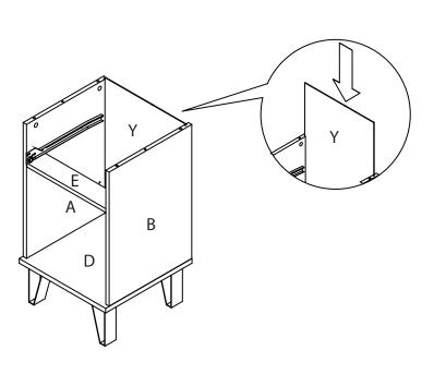
Insert the Back Panel (Y) along the slots on the Side Panels Right (B) and Side Panel Left (A).
