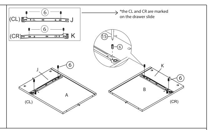
Attach the Drawer Slide CL (J) onto the Side Panel Left (A) and attach the Drawer Slide CR (K) onto the Side Panel Right (B). Then, use the Euro Screws (6) to screw the Drawer Slides to the Side Panel.
