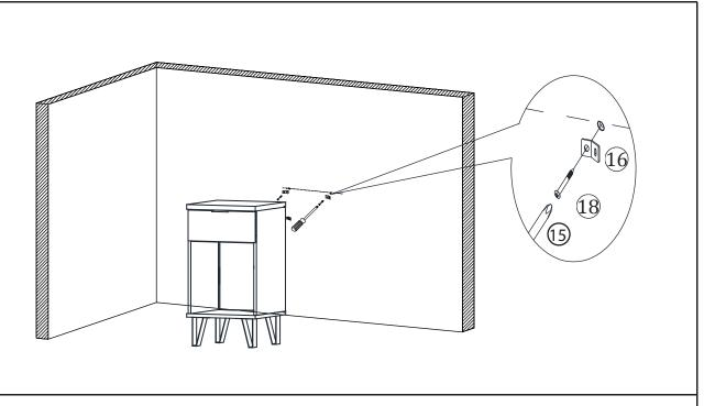
Attach the Metal Brackets (16) to the Wall Plugs(17) using Pan Head Screws(18) and a Screwdriver(15).
