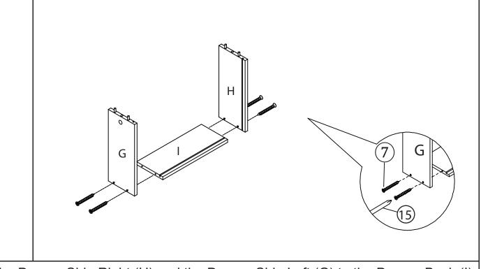
Attach the Drawer Side Right (H) and the Drawer Side Left (G) to the Drawer Back (I) using the Csk Screws (7) and the Screwdriver (15).
