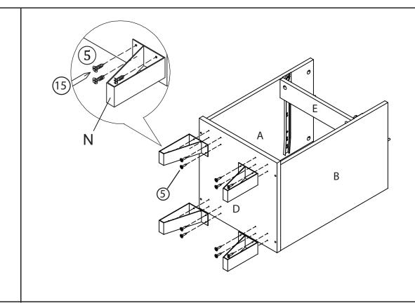
Follow the preholes at the Bottom Panel (D), attach the metal legs (N) and screw four Csk Screws ((5)) for each leg using the Screwdriver ((15)).
