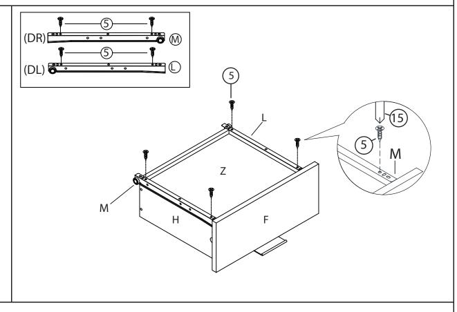
Place the Drawer Slide DR (M) onto the Side Drawer Right (H) and place the Drawer Slide slide DL (L) onto the Drawer Side Left (G) and secure them with two Csk Screws ((5)) on each side using the Screwdriver ((15)).
