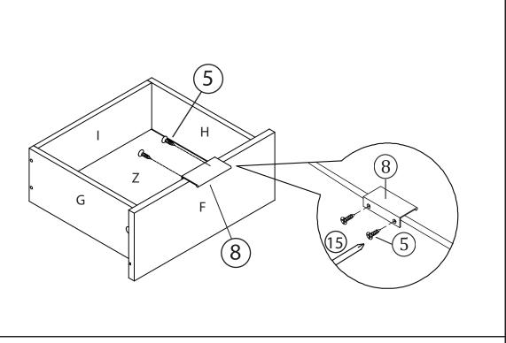
Follow the preholes, attach L-shape Handle (8) onto the Drawer Front (F) and secure with Csk Screws (5) using the Screwdriver (15).
