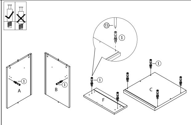
Attach Cam Bolt (1) to the mounting positions on the Top Panel (C) Side Panel Right (B) and Side Panel left (A) and the Drawer front (F) with a Screwdriver (15)
