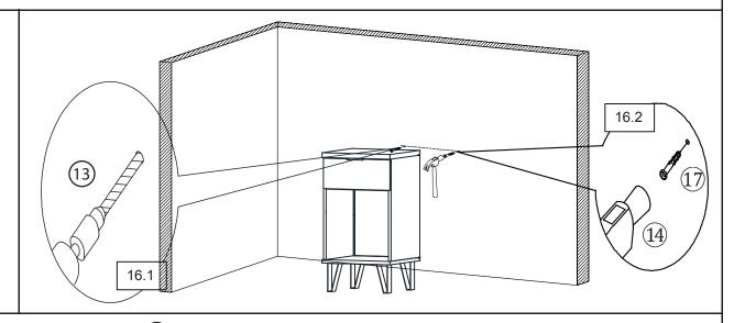
16.1) Using a Power Drill((3)), drill two holes into the wall at the same height as Metal Brackets((6)) that you have placed on the Tall End Table.
