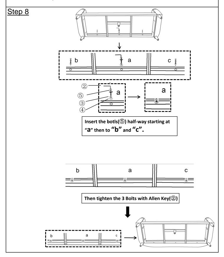
Secure Backrest(B) to the bottom of Seat Base(A) using Bolts( $\mathfrak{D}$ ), Spring Washers( $\mathfrak{D}$ ) and Washers( $\mathfrak{D}$ ) with Allen Key( $\mathfrak{D}$ ).
