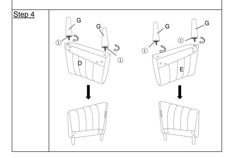
Carefully install the Wooden Legs(G) at the bottom of Left Arm(D) and Right Arm(E). Insert threaded stem into the mounting position at the corner of Left Arm(D) and Right Arm(E). Tighten by turning the Legs clockwise.
