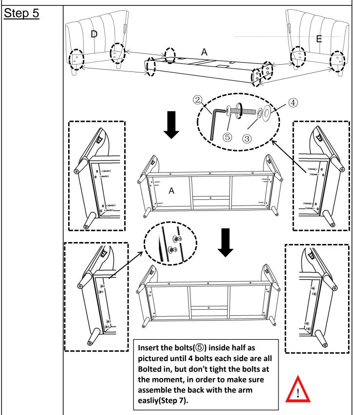
With assistance from your adult partner, postion Left Arm(D), Right Arm(E) and Seat Base(A) facedown on a clean, non-marring surface, then attach using Bolts(⑤), Spring Washers(③) and Washer(④) with Allen Key(②).
