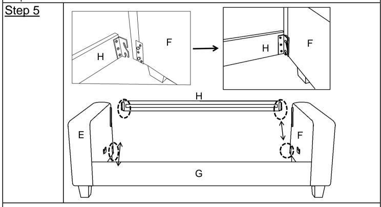
As to the Step 4, assemble the Hind Seat Board(H) at the behind of Left Arm(E) and Right Arm(F) as picture, don't need to tight with Allen Key.
