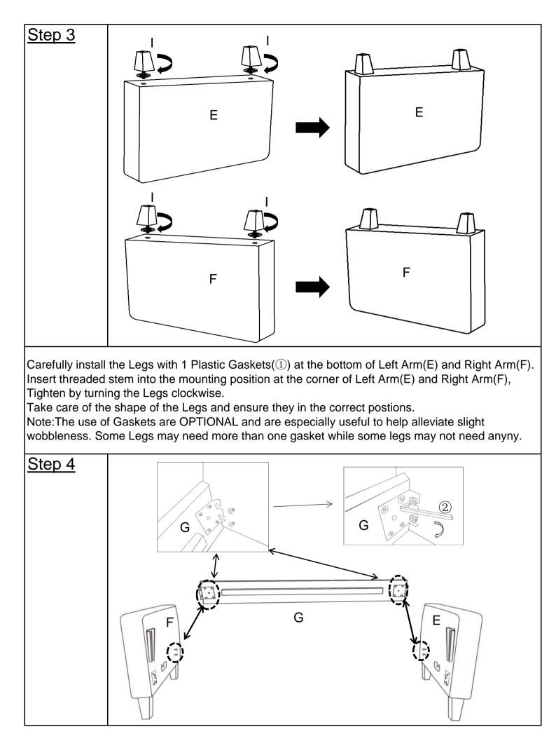
With assistance from your adult partner, postion the Left Arm (E) and Right Arm (F) as picture, hold up the Front Seat Board(G) and stand front the both Arms, assemble the Front Seat Board(G) by putting the metal hook on the two raised screws on the front side of both arms and push down make sure to the right position, then by tighten with Allen Key(2). do it one by one and make sure into position.
