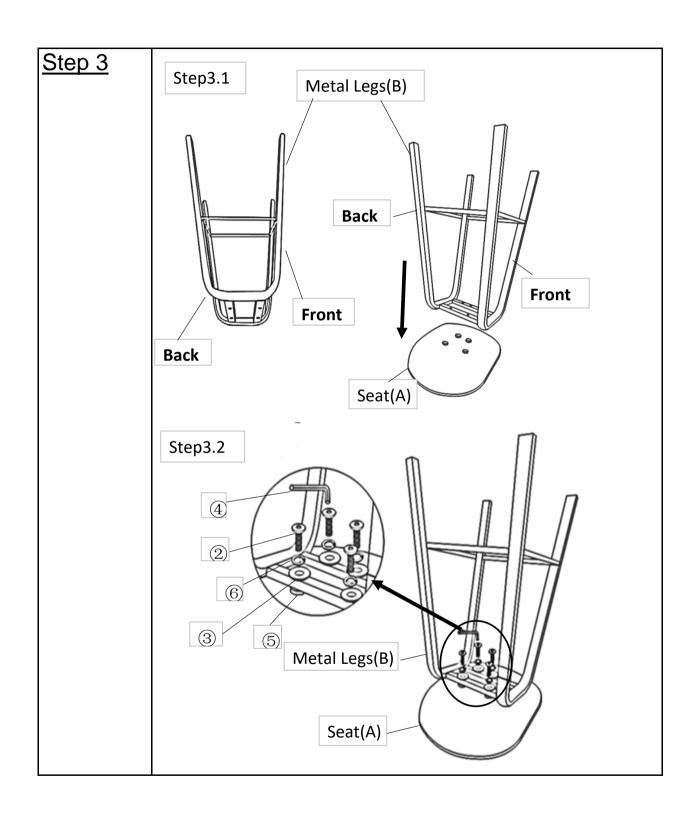
Step3.1 First, you must position the Metal Legs(B) lay on a clean, non-marring surface as shown on the left picture. Then you can find the angle of inclination of the back leg will be a little more larger than the front foot, as shown on the left picture.
