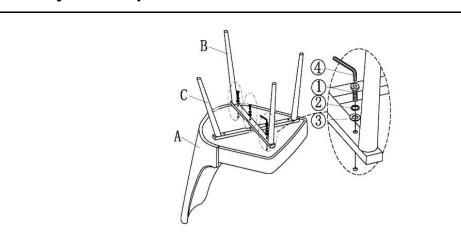
Attach Upper Leg Frame(C) to Lower Leg Frame(B), and Seat(A) using Bolts(1), Spring Washers(2) and Washers(3) with Allen Key(4) as shown above.
