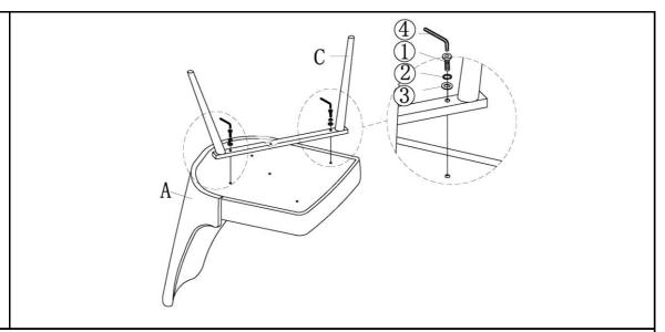
Attach Upper Leg Frame(C) to Seat(A) using Bolts(1), Spring Washers(2) and Washers(3) with Allen Key(4) as shown above.
