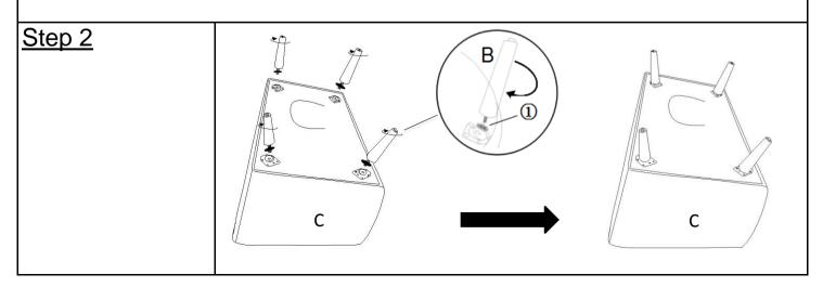
Install the Leg(B)at the bottom of the Sofa by placing one Gasket (①) on the threaded stem.
