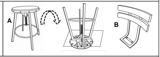
Put the parts on a clean, non-marring surface. Place the Seat (A) facedown onto a table, as shown.
