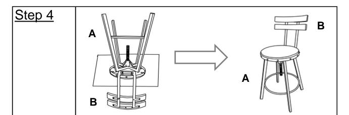
Stand the Barstool up and check the firmness of backrest, tighten all nuts.
