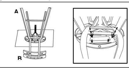
Align the mounting positions on the Seat(A) and the Backrest(B).
