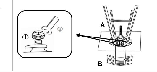
Attach Seat (A) to Backrest(B) using Nuts(1) with Wrench(2). CAUTION: When tightening these Nuts, tighten sequentially. DO NOT tighten any screw fully and then towards the next one.
